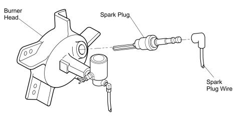
Figure 7 - Spark Plug Removal
